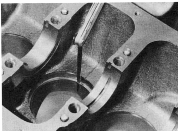
Check connecting rod bearing clearance
