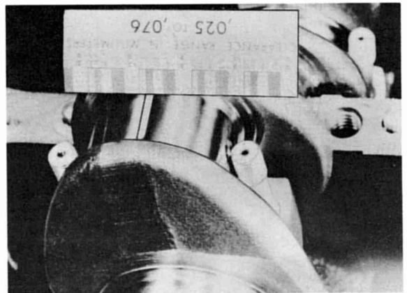
Check connecting rod bearing clearance
