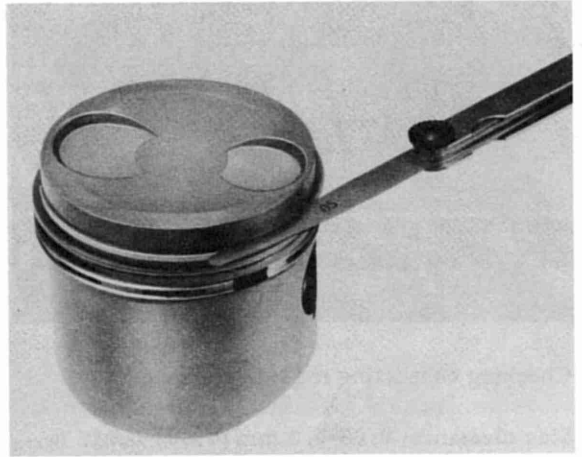
Check piston ring side clearance.
